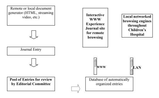
Figure 1 – EJ support software, architecture, and information flow.
