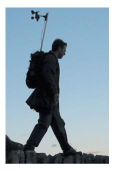
A sensor-equipped backpack detects wind, sunlight and moisture conditions around an outdoor trail. A handheld device shows the sensor readings along with changing locations as you hike. The suite includes Bluetooth, a Global Positioning System module, a compass, a sundial and maps. Narratives rendered in audio play at points of interest along the way.
